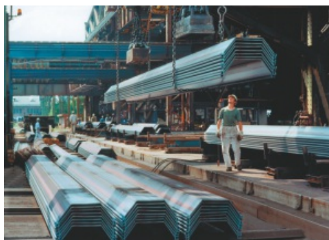
Spundwandlager Sheet pile stock
